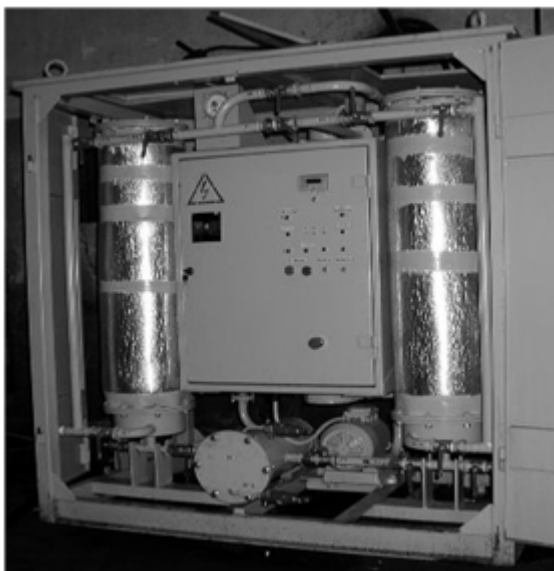
Fig. 4 – Industrial equipment for regeneration of transformer oil
