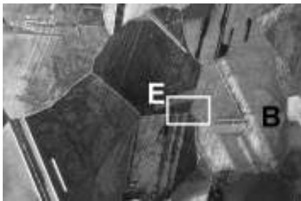
Figure 3 – Macroscopic image of original state of the annealed copper specimen.
