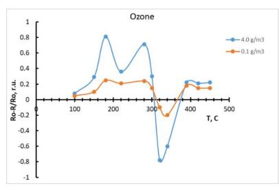
observed at temperatures of  $280^{\circ}$ C and  $330^{\circ}$ C, respectively, for an ozone concentration of 0.1 g/m3 and 4.0 g/m<sup>3</sup>. Moreover, S (O3) had a positive sign for a temperature of  $280^{\circ}$ C, and S (O3) was a negative value for  $330^{\circ}$ C.
